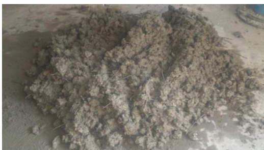
Figure 3. Concrete mixed with steel fibres
