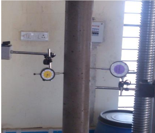
Figure 5. Extensometer connected over concrete column
