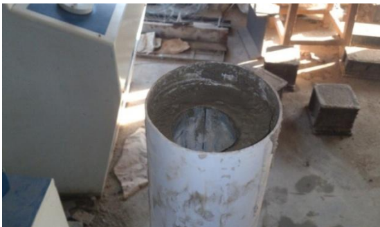
Figure 2. Column concreting using Hollow GI pipe
